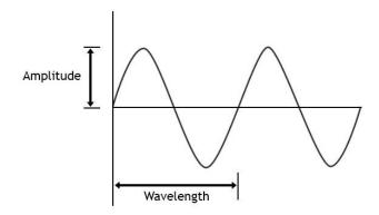
By definition, analogue forms must be continuous, ie have no break. We can say therefore that it has infinite resolution. (You can zoom in on the wave indefinitely and it will always be a continuous line with no gaps in it.)
